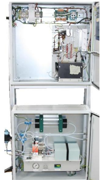
Fig. 10 PSA 10.216 Workroom Air monitor configured for sequential testing of elemental and oxidized Hg generators.
