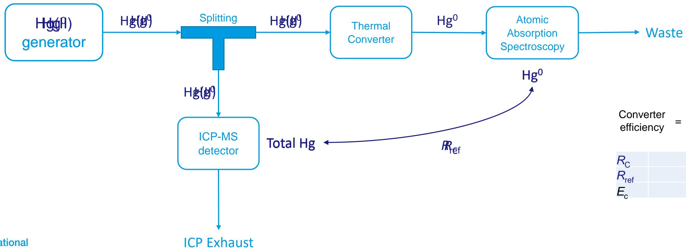
$$\text{Converter efficiency} = \frac{R_C}{R_{\text{ref}}}$$
