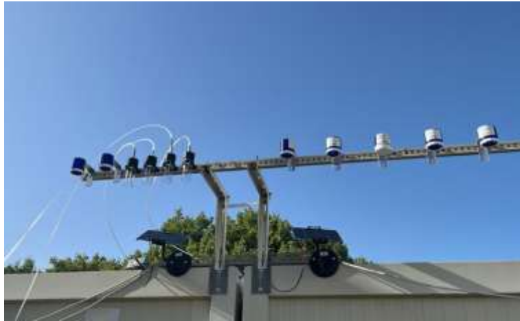
Figure 17. Deployment of the remote tube samplers on the rooftop of the monitoring station
