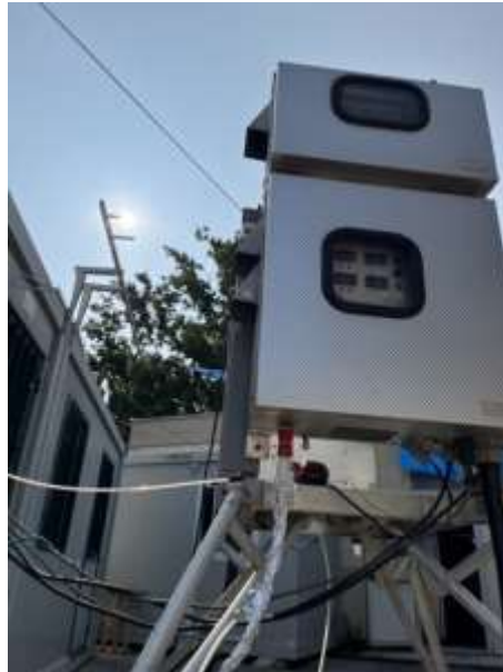
Figure 4. Tekran Speciation Units System with aluminum-coated sample line
