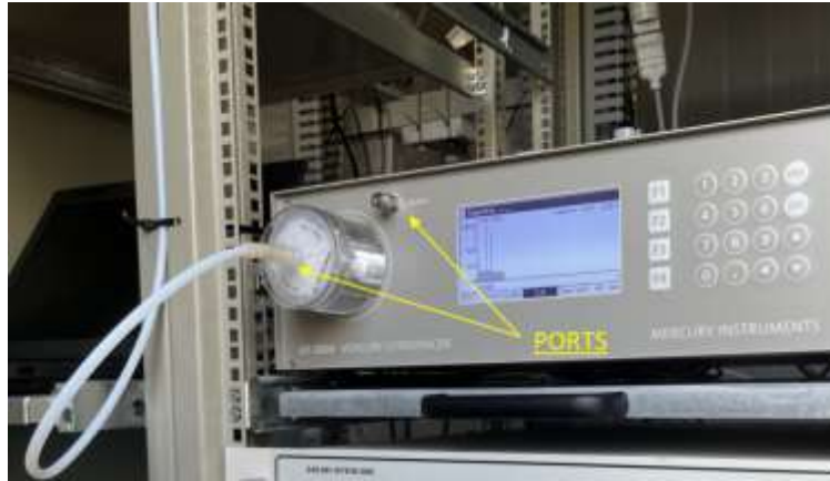
Figure 13. UT-3000 sample line and injection port used for calibrations
